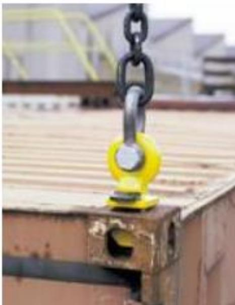
**Figure 1: Typical top lifting lug (yellow)**
